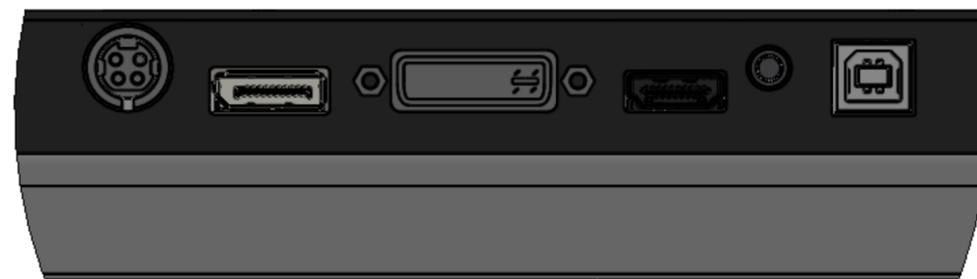
**Inputs:** DC Power, Display Port, DVI, HDMI, Audio In, USB Type B\*
